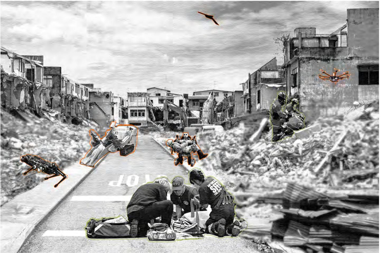
Figure 1. Human machine teaming scenario for disaster search, rescue, and recovery operations. Autonomous robotic systems work collaboratively with humans to search for survivors (high altitude, fixed wing drone, top; hover drone, right; land scout, left), and transport wounded (walking robot carrying injured, center-right; bed transport, center-left).
