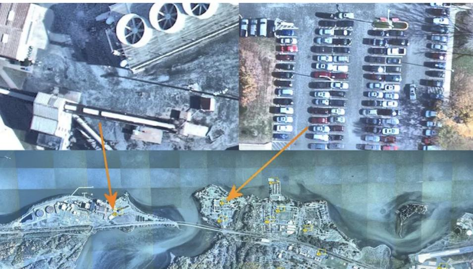
Part of a DARPA ARGUS-IS image of Quantico Marine Corps Base in Virginia (2nd row), with two targeted areas illustrating the six inch resolution of the camera (1st row). (image courtesy of DARPA)
