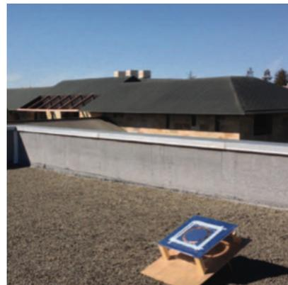
**Figure 2. (Left) Solar steam generation by heat localization (Ghasemi et al. Nat. Comms 5, 4449 (2014)). (Right) Passive radiative cooling under direct sunlight (Raman et al. Nature, 515, 7528 (2014)).**
